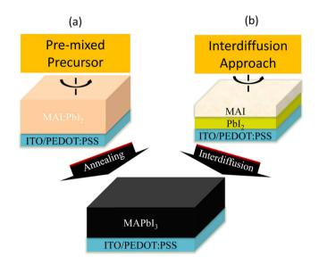
**Figure 1.** Schematic of the prepation of perovskite films by (a) spin coating of pre-mixed precursor of lead iodide  $(PbI_2)$  and methylammonium iodide  $(CH_3NH_3I)$  and (b) an interdiffusion approach. ITO: Indium tin oxide, a transparent conducting oxide. PEDOT:PSS: A transparent, conductive polymer. MAI: Methylammonium iodide. MAPbI<sub>3</sub> Methylammonium lead iodide.
