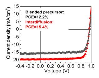
**Figure 2.** Photocurrents of the devices under standard 'AM 1.5' simulated illumination with perovskite films fabricated by the blended precursor solution and interdiffusion methods. PCE: Power conversion efficiency.
